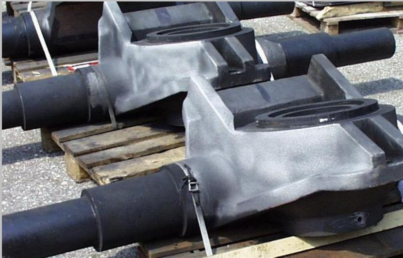
Pendulum of a bowl mill, protected by ArC metal spraying
