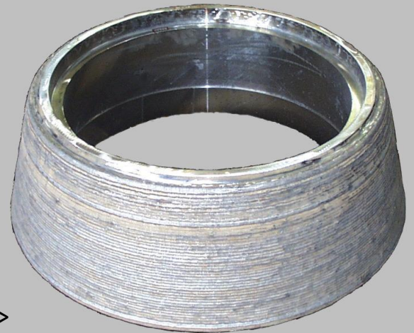
Mill liner protected by ArC metal spraying →
