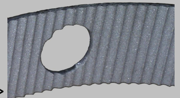
Mill liner protected by ArC metal spraying →
