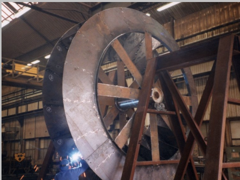
Ventilator: blade wheel with A.S.S. plates
